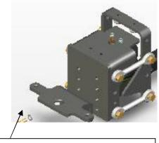
Insert 4 Bolts to Ball Mounting Plate and torque at least to 55ft-lbs and not to exceed 100ft-lbs.
