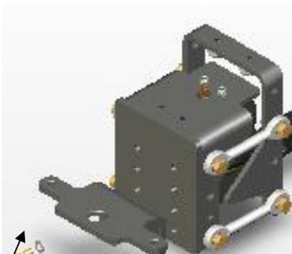
Insert 4 Bolts to Ball Mounting Plate and torque at least to 55ft-lbs and not to exceed 100ft-lbs.
