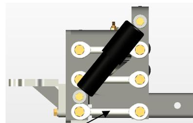
Ensure Tie Rods are Level for proper ride height
