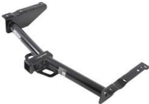
The trailer hitch attaches to the frame of your vehicle and provides the 2" x 2" (or 2-1/2" x 2-1/2") receiver opening that the weight distribution shank slides into. Trailer hitches are classified based on weight-carrying capabilities. A trailer hitch must be categorized as Class
